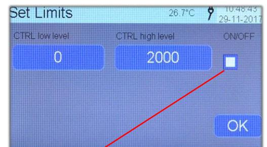
In the example the upper threshold is set to 2000 Pa. In the set value input mask appears the reduced input range of 0...2000 Pa. Without activated ON/OFF button, the nominal range of 0...7000 Pa of the corresponding module appears.
